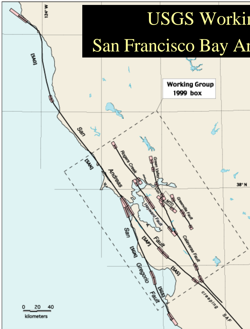
Figure 0.1. Dashed rectangle (Working Group 1999 box) shows the region included for calculation of earthquake probability and seismic moment. Bold solid lines indicate major faults for which probabilities were calculated. MTD, Mount Diablo Thrust; Con, Concord Fault.
